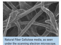
Media is, of course, the main factor influencing pressure drop; indeed, it causes pressure drop. That's why having a low-friction, high-flowing media is so important. The natural cellulose or
