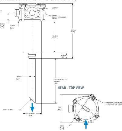
Max Flow: 150 gpm (568 lpm)
