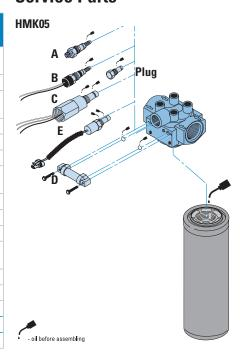
Filter Notes: Refer to table in the Technical Reference Guide for fluid compatibility with our filter media. Thread size is 1 3/4\*-12 UNF-2B.
