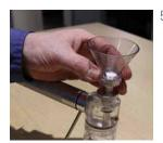
5. Reattach the funnel to the filter patch base with filter patch. Twist lock the funnel to the base.
