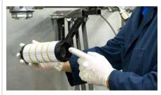
Install filter into the housing.
