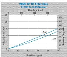
Max Flow: 200 gpm (757 lpm)
