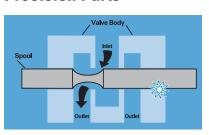
This illustration of a simple hydraulic valve illustrates how particles damage components. In normal operation, the spool slides
