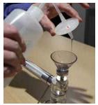
8. Once the entire sample has passed through the patch rinse the funnel with filtered solvent and draw through the patch. Continue to pull air through until the patch starts to dry. Then separate the funnel from the patch supporter and remove the patch with forceps.
