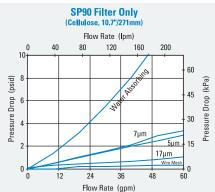
Max Flow: 100 gpm (379 lpm)
