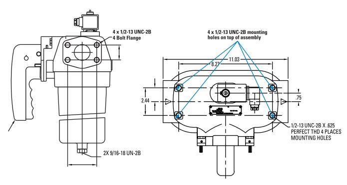
Max Flow: 100 gpm (379 lpm)
