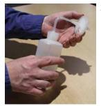
2. Install solvent\* dispensing tube and install solvent filter on end of the dispensing tube.
