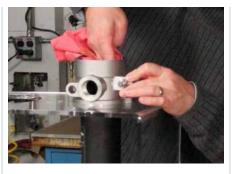
Wipe away any sediment on the outside of the filter cover.
