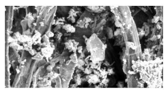
Excessive dirt in the media can cause dirt migration or even filter failure. Dirt migration occurs when the restriction is so great that the differential pressure pushes dirt deeper into the media and, eventually, through the media and back into the system. Filter failure occurs when the restriction becomes so high that the filter cartridge collapses (outside-in flow) or bursts (inside-out flow) to relieve the upstream pressure.
