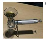
6. Agitate the sample fluid bottle and pour 25ml into the funnel, 25ml is denoted by the first line on the funnel (closest to the patch).
