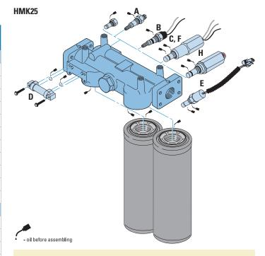
Lubricate filter-to-head threads when installing new filter to prevent thread damage. Heavyweight gear lube is recommended.
