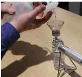
3. Rinse the funnel-patch assembly with the filtered solvent to remove background contamination. The patch should not be in place for this process.
