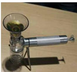
6. Agitate the sample fluid bottle and pour 25ml into the funnel. 25ml is denoted by the first line on the funnel (closest to the patch).
