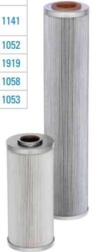
All Donaldson DT filters utilize glass fiber media with an epoxy-based resin system for the ultimate in chemical compatibility and are potted with epoxy-based adhesives. Standard collapse designs are double wire-backed using epoxy-coated steel mesh for maximum pleat support and dirt capacity. Fluorocarbon seals are standard on all Donaldson DT filters.
