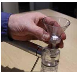
5. Reattach the funnel to the filter patch base with filter patch. Twist lock the funnel to the base.
