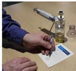
9. Place the sample (ink/dirty side up) on a clean index card and cover it immediately with a plastic laminate patch cover.
