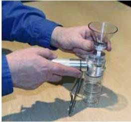
1. Assemble waste bottle, funnel-patch assembly, and vacuum pump to form the sample processing assembly. Tighten the vacuum pump o-ring on the funnel-patch assembly tube by turning the aluminum locking device.
