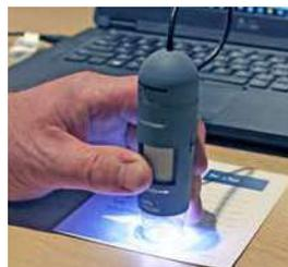
11. For best results, stand the microscope (without the lens cap or base) directly over the sample.
