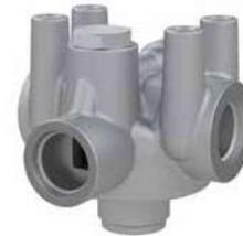
The P167529 head is designed with a 50 psi / 3.45 bar third port bypass valve that diverts all bypass flow back to the reservoir, instead of going straight through the head and into the system as it does in 2-ported heads. Unfiltered fluid is NOT allowed into the system in the case of plugged filters. Designed primarily for charge pump applications.
