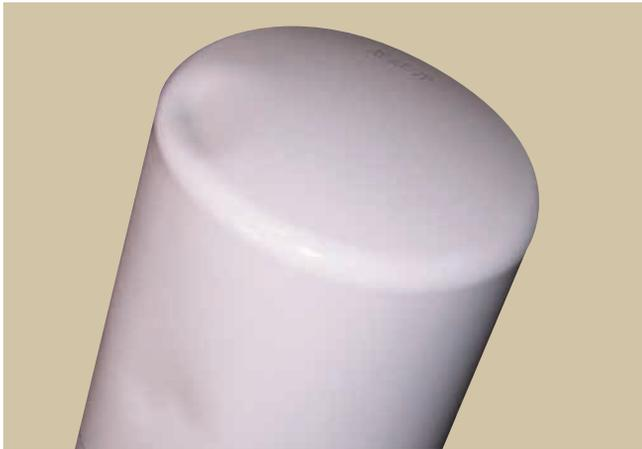
Dents in a steel filter canister create a concentration of stress—making the canister more susceptible to fatigue.
